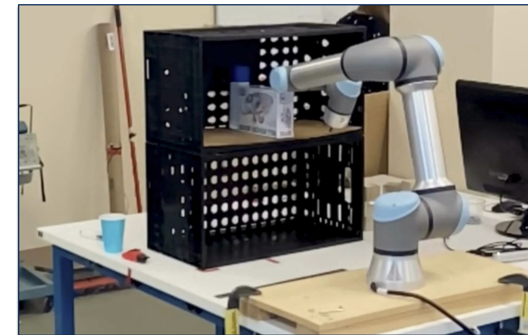
Figure 3: Setup for UR5e experiment with shelf
